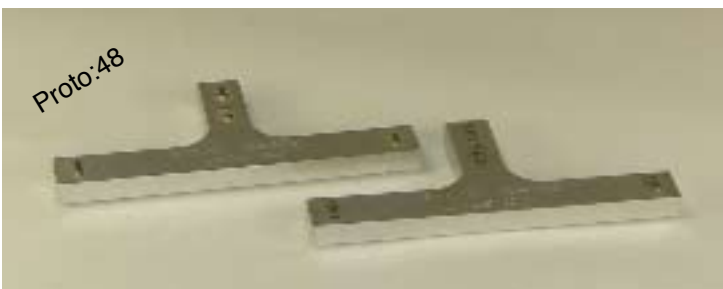
Track laying gauge - Code 100 - Code 125 - Code 138 designed by Paul Martineau
