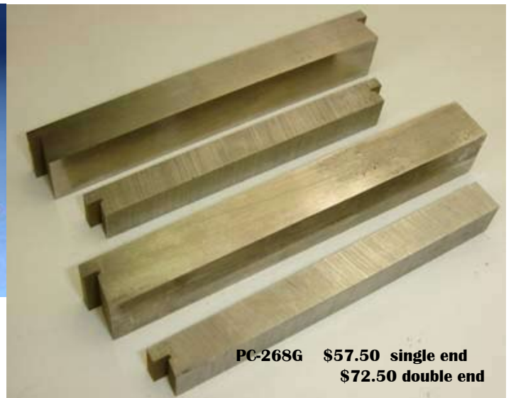
Proto:48 contour form tool made from M-2 hardened tool steel. AAR 1/48 profile dimensions: .115" x .0257" flange, fillet and 20:1 taper. Available in 3/8" or 1/4" shank.
